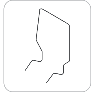
Preformed wire clip 38 mm Galvanized mild steel wire
